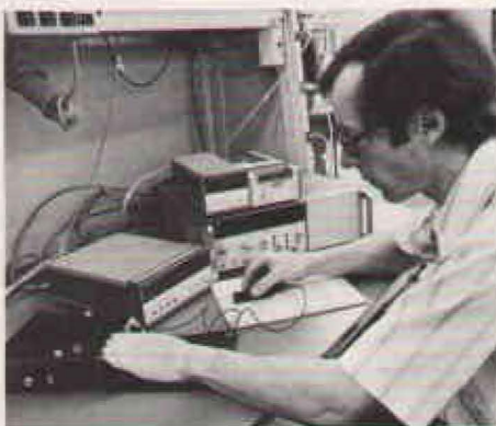
Art Lange shows how a blind person would read with his hands using the Optacon. The "ASCII to Optacon Interface" (center) connects to the test instruments at right.
