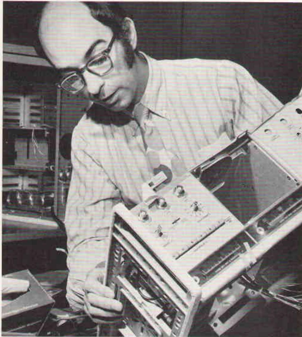
Nearing end of production line at South Queensferry where it was developed to become an international success, a microwave link analyzer (MLA) is checked by line supervisor Jim Stewart.
