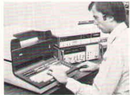
At left is the 3050B automatic data acquisition system from AMD, representing usage in a standard-type system, one which uses a scanner with multimeter and calculator for a low-cost solution to data gathering and data reduction.
