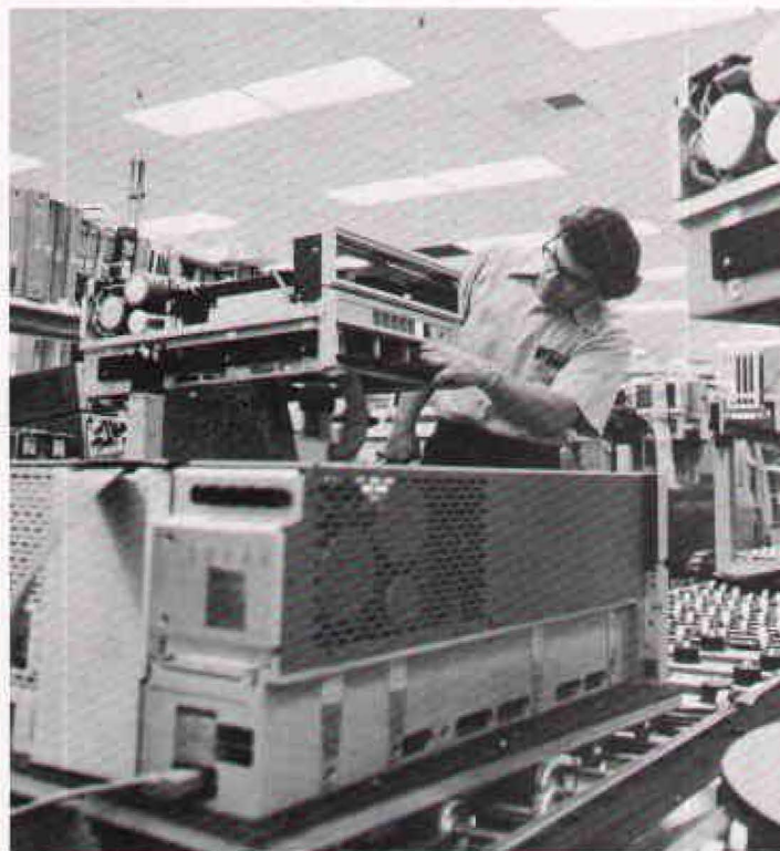
Rob Crumb checks out a 7905A disc drive in the initial diagnostic test area.
