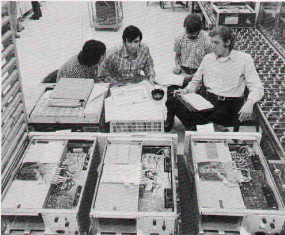
Lead Bernie Appleby (left) explains critical environmental test procedures in HP-21MX and HP-2100 manufacturing area at Cupertino. Minicomputers are put through extensive temperature and humidity tests before being shipped. Undergoing training (from second to left) are Jay Hendon, Steve Bissell and Dave Dillon.
