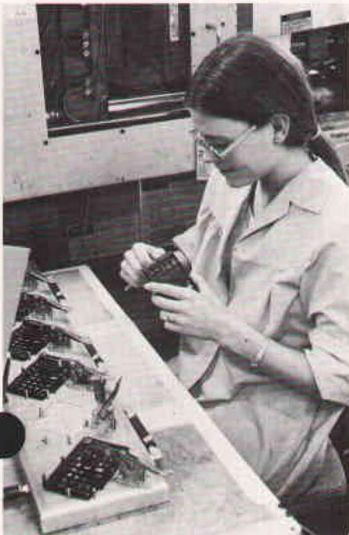
*HP has emerged as a leader in plastics-molding technology, especially since tackling the requirements for complex cases for hand-held calculators, and two-color moldings for keyboards. To achieve high levels in precision, specialists from both the plastics-molding and tool-and-die departments work closely with product designers in the client divisions. Here operator Joan Imschweiler checks two-color molding of an HP-65 keyboard.*
