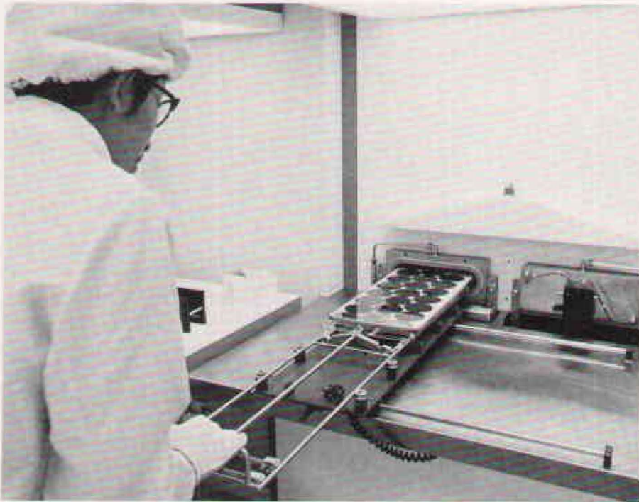
Henry Chiang of HP Labs puts a batch of IC wafers through one of many process steps — in this case to add a dielectric material. This laboratory on Deer Creek Road in Palo Alto is the newest and most automated IC facility in the company.
