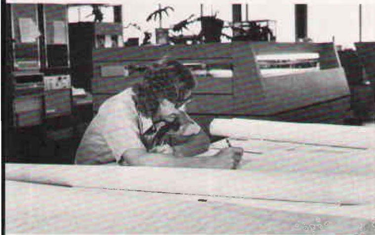
Design engineer Lou Scheffer of Loveland (Colorado) Instrument Division checks an IC drawing made on the large horizontal plotter in the background. Most HP divisions use similar computer-aided artwork (CAA) systems to simplify the job of drafting complex circuitry.
