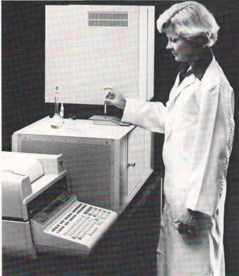
Entering sample in an HP 5992B GC/mass spectrometer.
