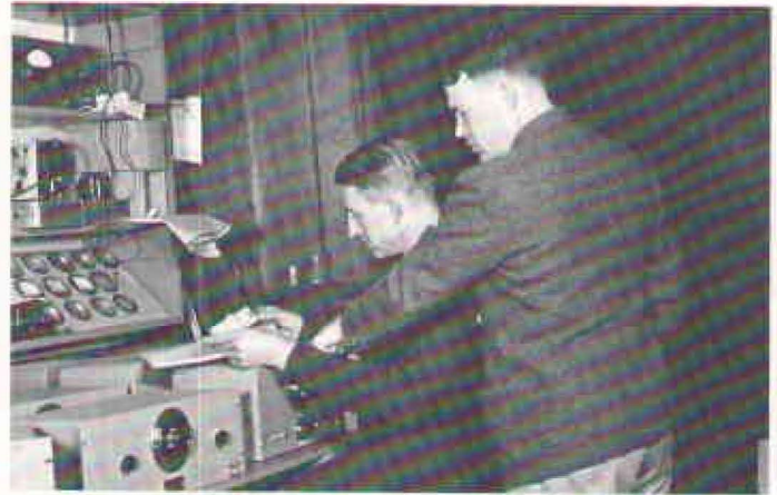
In this early photo taken in the garage, Dave Packard (seated) and Bill Hewlett run final production tests on a shipment of 200A audio oscillators, the product that put them in business in 1939.
