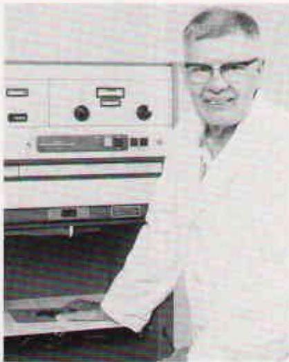
The HP Faxitron 43805 was the "camera" used by Al Duggan of the McMinnville Division to make the X-ray pictures on these pages. (For photography buffs interested in details, he used an Eastman 8x10 LP4 graphic-arts film for his negative, then increased or decreased the contrast as necessary during development).
