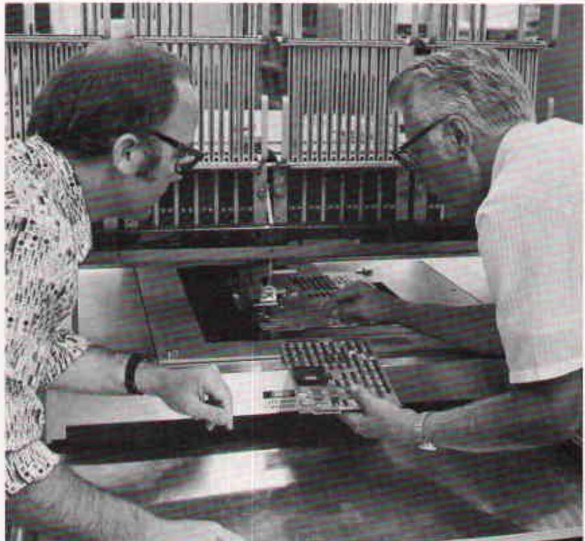
Checking the installation of a new automatic PC board loading machine at Data Systems Division are Gaylan Larson, manufacturing manager at left, and Wally Johnson, supervisor of the board-loading area. Automation was made economical largely through standardization of board sizes.
