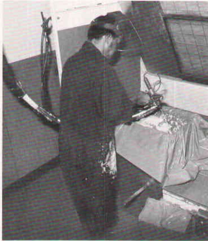
Plastic slurry is carefully injected into mold where it foams up and hardens to create a highly protective package at lower cost for shipment of San Diego products.
