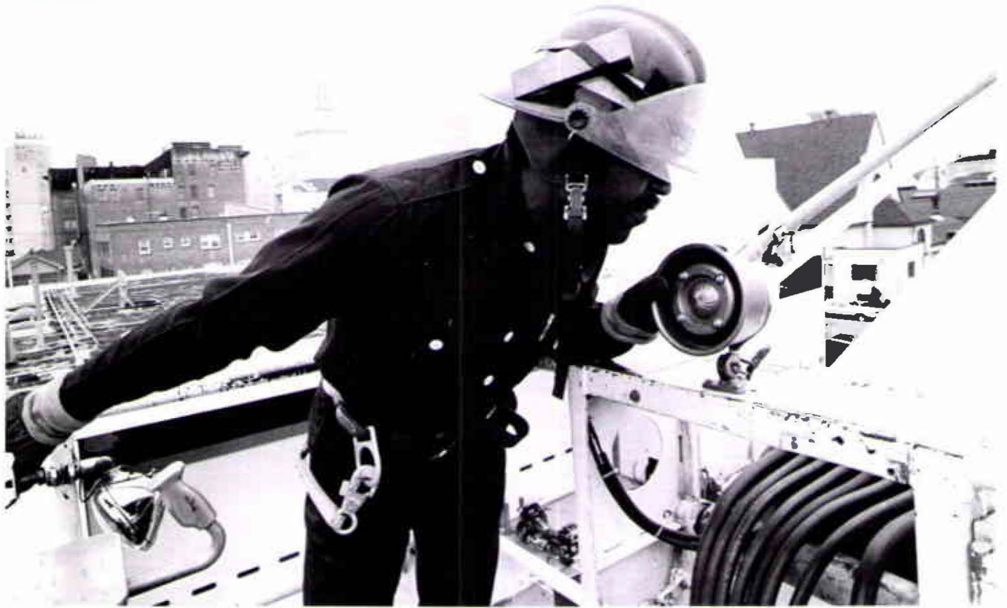
Charles Gardner operates the "snorkel" that lifts firefighters as high as 85 feet in the air at emergency scenes.
