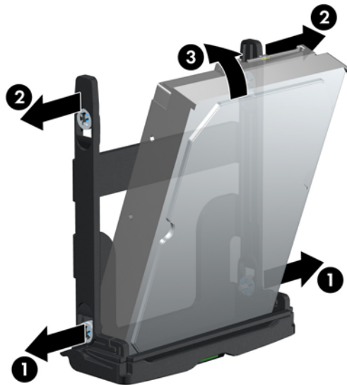
Figure 9-5 Installing the drive in the carrier
