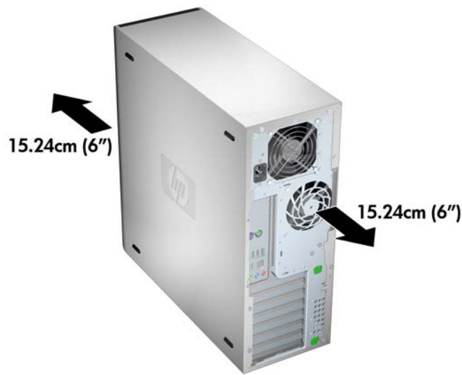
Figure 3-1 Proper workstation ventilation
