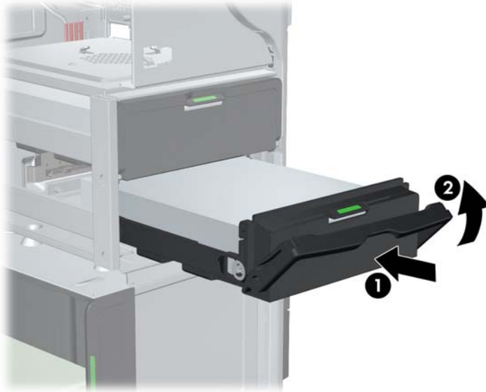
Figure 9-6 Installing the HDD in the chassis
