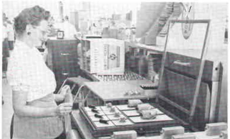
Skin packaging equipment was first installed at HP in 1960 and has since proved a big money saver for protecting small items. Ginger Bradley is shown holding polyethylene film which is lowered over group of components, then heat-sealed skin-tight.
