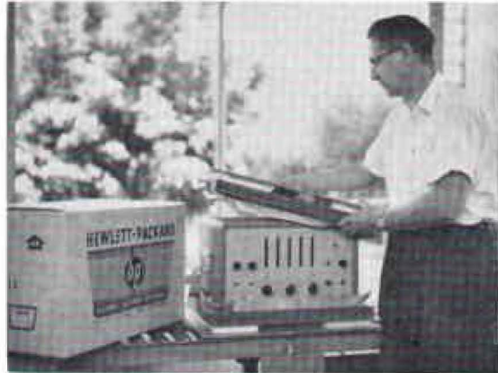
Harry Wood shows inside elements of the highly successful floater package. The two pads, which fit the instrument top and bottom, permit floating action vertically and horizontally (or technically, in shear as well).
