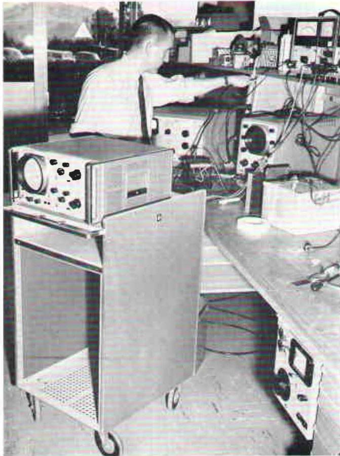
New Testmobile, a general purpose test cart, can accommodate any HP instrument. Gerry Priestley, Dymec industrial design engineer, shows how instruments can be wheeled to within arm's reach of technician at typical bench position.
