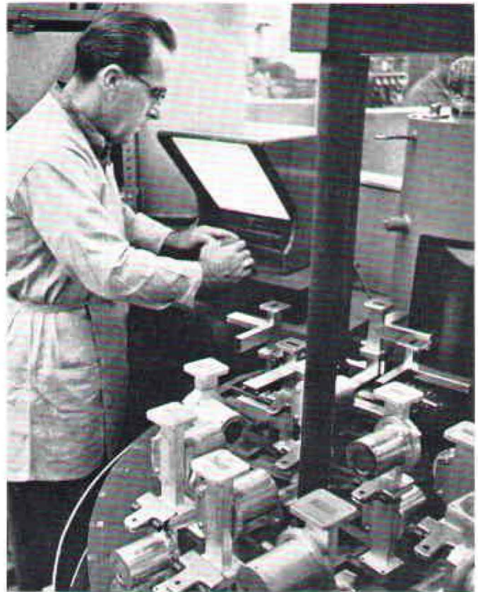
Lapping Specialist Nino Bandino of the Stanford plant's waveguide machine shop is seen at the monochromatic light projector where wheel surface readings are taken with an optical flat. A lapping machine, loaded with waveguide assemblies, is partially shown at right. Flanges can be ground to accuracies of eleven millionths of an inch.
