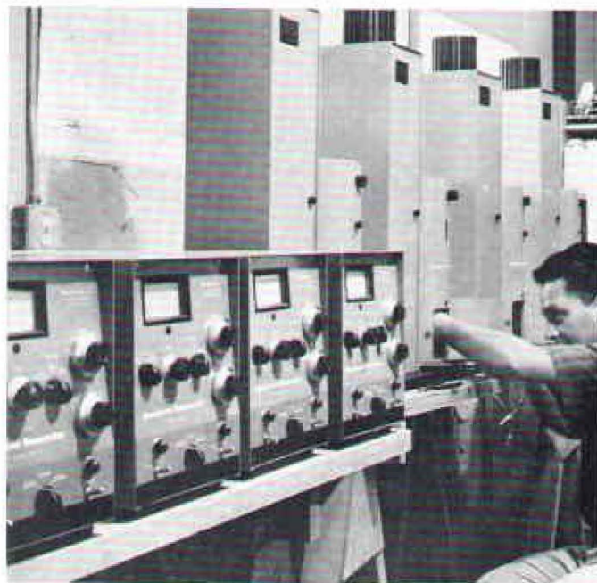
Assembly of four membrane high-speed osmometers nears completion. Instruments determine molecular weights of substances.
