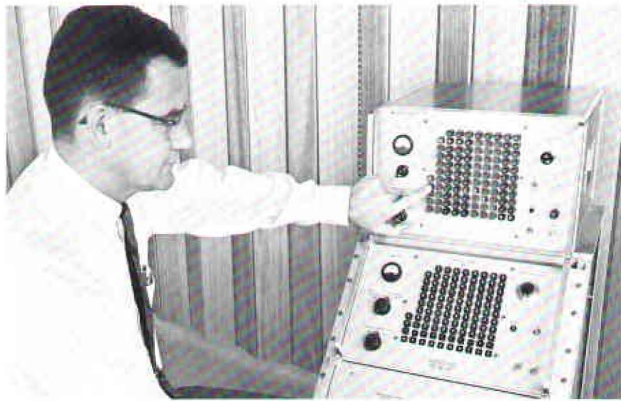
Product design engineer Ted Pichel shows how new pushbuttons light up on a frequency synthesizer.
