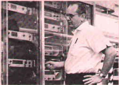
Manufacturing quality plus rigid testing and control have built highest reputation for F&T products. Here test line leader Dave Keller inspects group of 5245 counters being operated under elevated temperatures.
