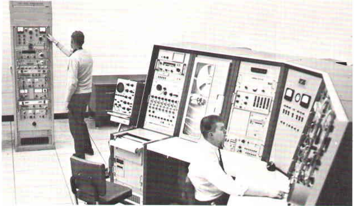
Telemetry and command console (foreground) is seen during checkout by Early Bird simulator. Majority of instruments in the simulator (rear) were produced by HP divisions. In addition, a Boonton FM-AM signal generator is used as modulator/transmitter for TV sound channel at Andover.
