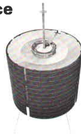
The Early Bird satellite (above), built by Hughes Aircraft, is powered by 6,000 solar cells. The giant horn reflector (below) at A.T. & T.'s Andover ground station is tremendously sensitive to satellite signals.
