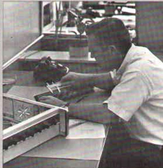
Here Rich Hoogner checks a cardboard mock-up of a proposed instrument readout panel.
