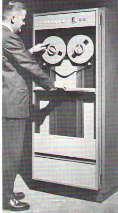
Model D 3030 magnetic tape units were designed by Datamec for medium speed computer market.
