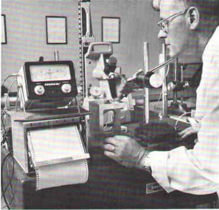
Glenn Herreman makes a thin film measurement with ingenious system developed by gage lab using a Moseley strip chart recorder.
