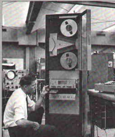
A Dymec digital data plotting system with a Data-mec tape transport is tested by Jim McCabe.
