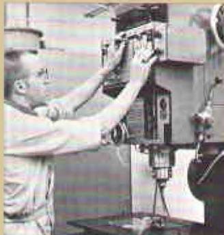
Precision drilling is done in machine shop by this tape controlled equipment, shown here being set up by Peter Penninga.
