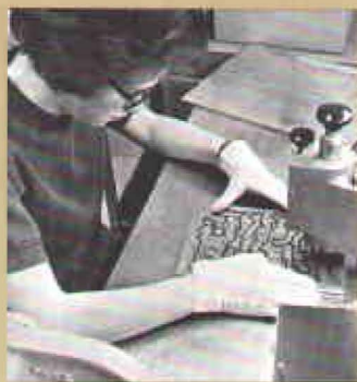
As one stage in the production of printed circuit boards, Charmene Arajakis drills holes to accommodate components.
