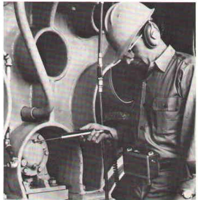
Using a Delcon ultrasonic translator detector, mechanic checks Crown Zellerbach paper mill for faulty bearings.
