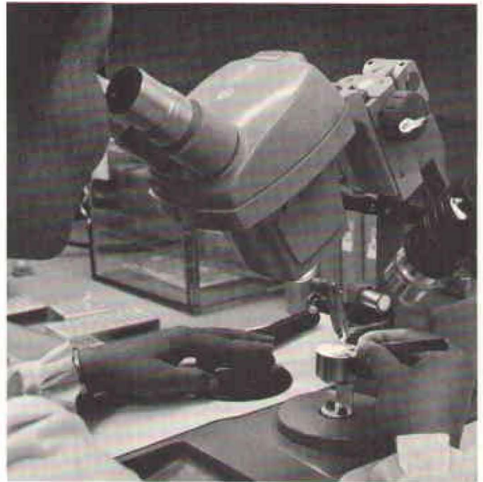
Using gossamer-thin aluminum wire, microscopic connections are made by ultrasonically joining points on an IC chip to the frame. At the controls is F&T's Frances Hartman-Kok.
