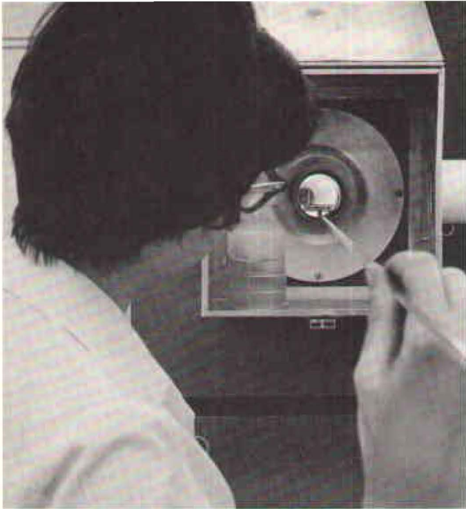
Sharon Martin inserts a "boat" of IC wafers into furnace that treats them at high temperature, one of several major steps in creating finished chips on surface of a silicon wafer.
