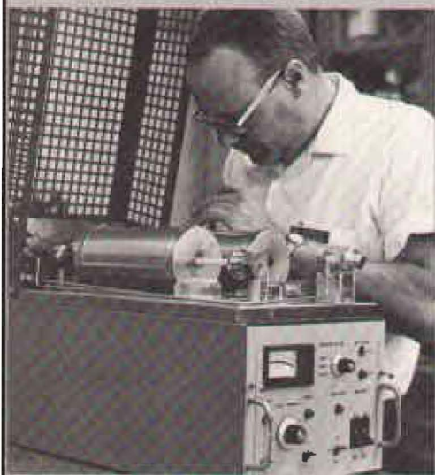
Newly developed Redox unit is checked by Howard Ashmead, supervisor of elemental and macromolecule section. Device can be added to Model 185 analyzer to enable it to check for oxygen and eventually for sulfur in addition to carbon-hydrogen-nitrogen tests.
