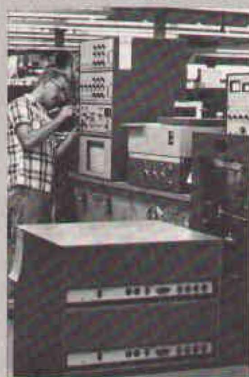
Final test on Model 402 high efficiency chromatograph is made by test technician Jack West. All instruments are put through rigid check-out procedures before shipment to customers.
