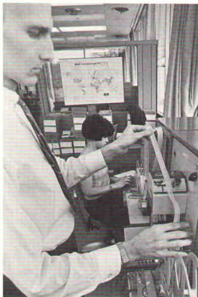
Messages received from Europe via high-speed punched tape are screened in Rockaway by Joe Chaston. Rockaway and Palo Alto are both distribution points for European messages to divisions in the U.S. Known as DATEX, the system transmits 1,200 words a minute.
