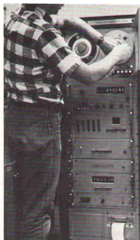
Measurements of the chemical nutrients in seawater once done by hand at Scripps Institute of Oceanography's Institute of Marine Resources now speed through an HP 2010H data acquisition system.
