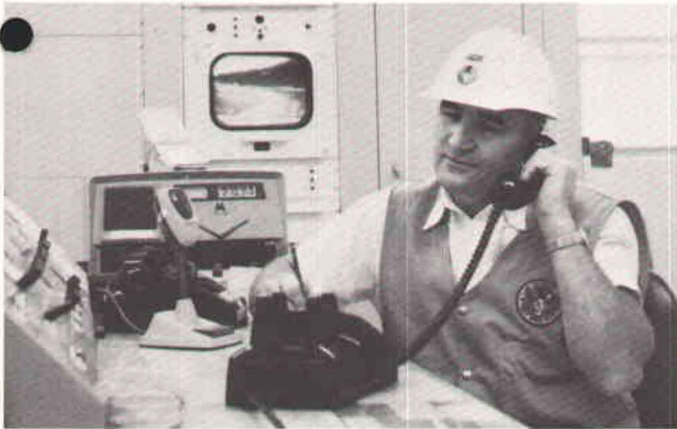
The coming era of the totally automated highway is beginning to show itself in a number of electronically instrumented traffic control systems now being used in and near large cities. Typical is this lane control installation in which monitor at left observes traffic on closed-circuit TV then automatically changes sign at right to give drivers warning well in advance.
