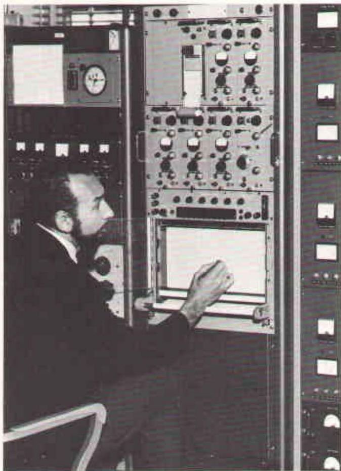
Radio signals from the sun are subject of intense study by astronomers at Penn State. Dr. Ray Vogt, above, uses HP 6-channel recording oscillographic system as well as data acquisition system. At right, Stanford University radio astronomer Ned Conklin examines waveform of a pulsar on prototype HP signal averager which served to eliminate unwanted radio noise.
