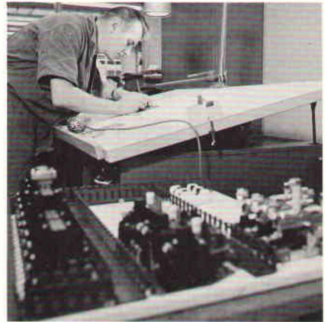
Erich Jurak, a machine rebuilder with extensive training in electrical engineering, draws schematic for automating Wiedemann punch press machines. In the foreground are components which machine services will install in the equipment.
