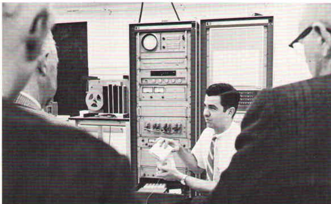
The HP 9500A automatic test system, demonstrated for visiting customers here by Dawson Mabey, is Systems Division's new and versatile entry into fast-growing test systems market. The 9500A employs a wide range of standard and optional HP instruments.
