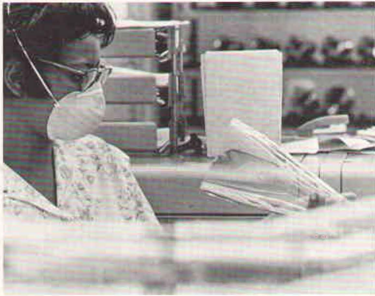
Among efforts to improve CRT quality was a worldwide search for superior glass. Here Jean Jones checks effect of heating — “fritting” as it is known in the trade — on a storage tube funnel. Face mask is worn to protect super-sensitive CRT.
