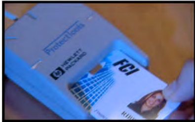
Figure 2 Logging on with a Smart Card
